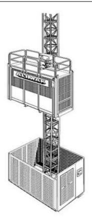
The Alimak Scando 650 Passenger/Goods Hoists can be used in single or dual configuration. The hoist cage design is truly modular and offers several optional cage lengths between 3.2m - 3.9m and 3.9m - 5m. depending upon the required capacity, the cage will be fitted with the two or three VFC frequency controlled motors or two direct online motors which drive the system through high efficiency gearboxes.
